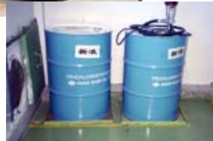
Pans set under all drums containing trichloroethylene fluid to prevent its leak (Jiangsu Mabuchi)
