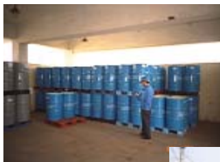
Leak-proof and explosion-proof storage for storing chemical substances including wash agent (Jiangsu Mabuchi)
