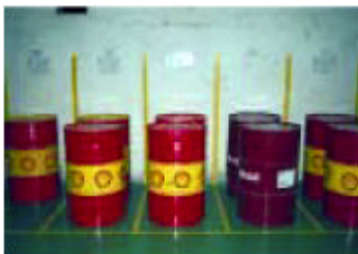
Floor coated to prevent liquid spill (Dalian Mabuchi)
