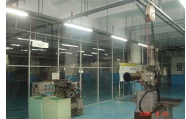
The number of transparent plastic screens was increased to improve air conditioning (AC) efficiency. That reduced consumption of electricity for AC and lighting without affecting visibility (Guangdong Mabuchi)
