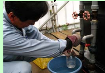
Decontaminated groundwater is sampled periodically to examine its quality.
