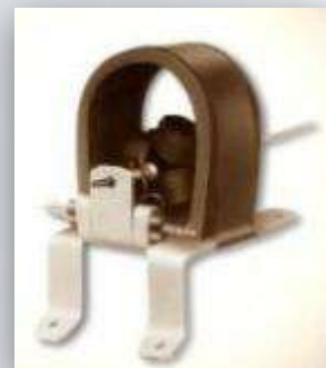
Horseshoe-shaped magnet motor that the founder invented in 1947
